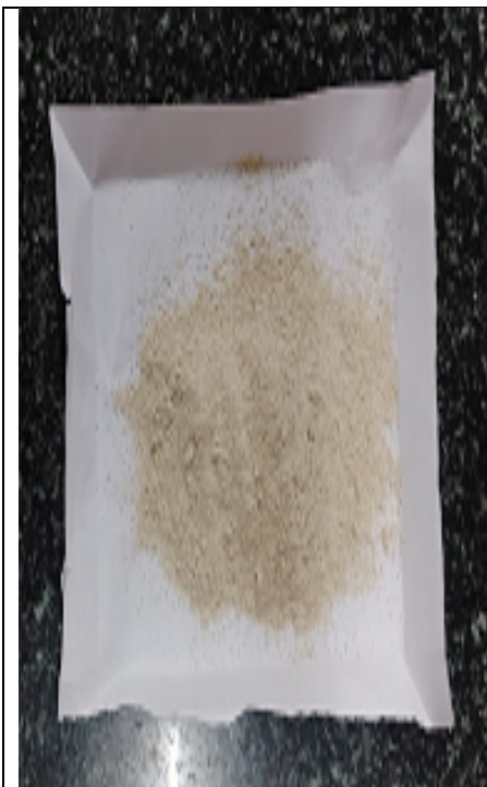
Fig- 2.1 Preparation of banana starch from banana peels
