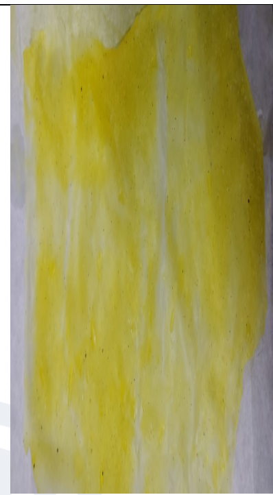
Fig- 2.2 B Production of bio-plastic using sorbitol as plasticizer
