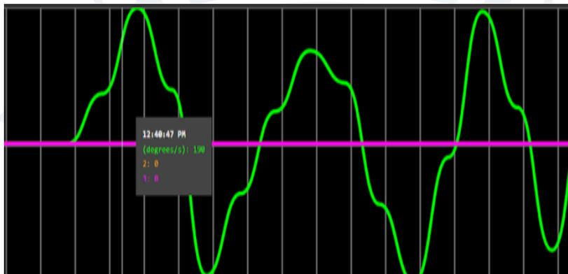
Fig 10: Gyroscope of MPU-6050 Along Positive X-Direction
