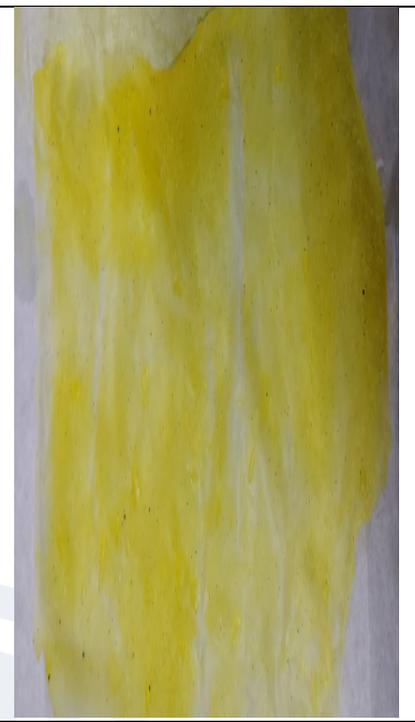
**Fig- 2.2 B Production of bio-plastic using sorbitol as plasticizer**
