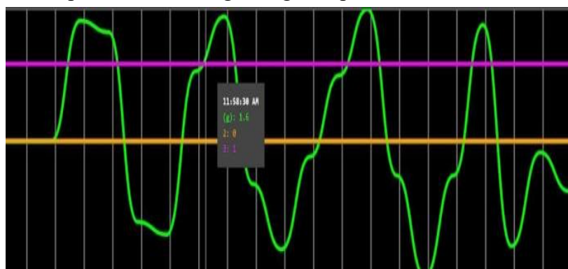
Fig 6: Acceleration Of MPU-6050 Along Positive X-Direction
