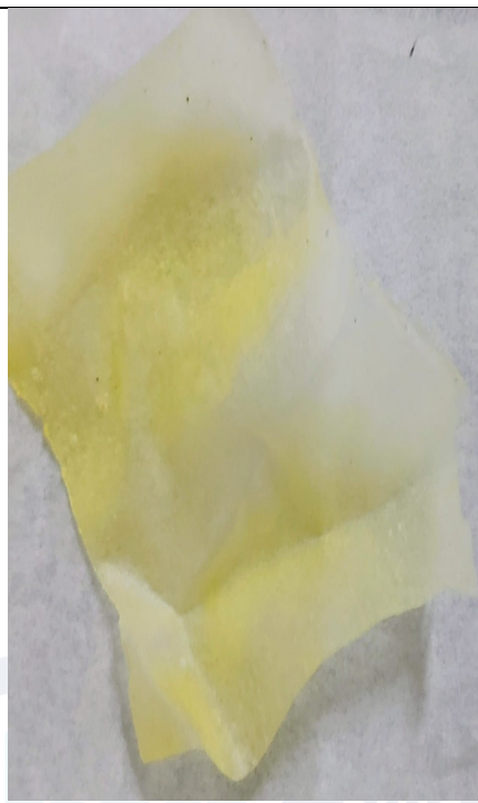
Fig- 2.2 A Production of bio-plastic using glycerol as plasticizer
